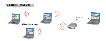
In Client mode, the Travel Router is connected to the Ethernet port of your PC (or other device), and will connect to a Wireless LAN. This has the effect of converting the Ethernet port to a Wireless interface.
